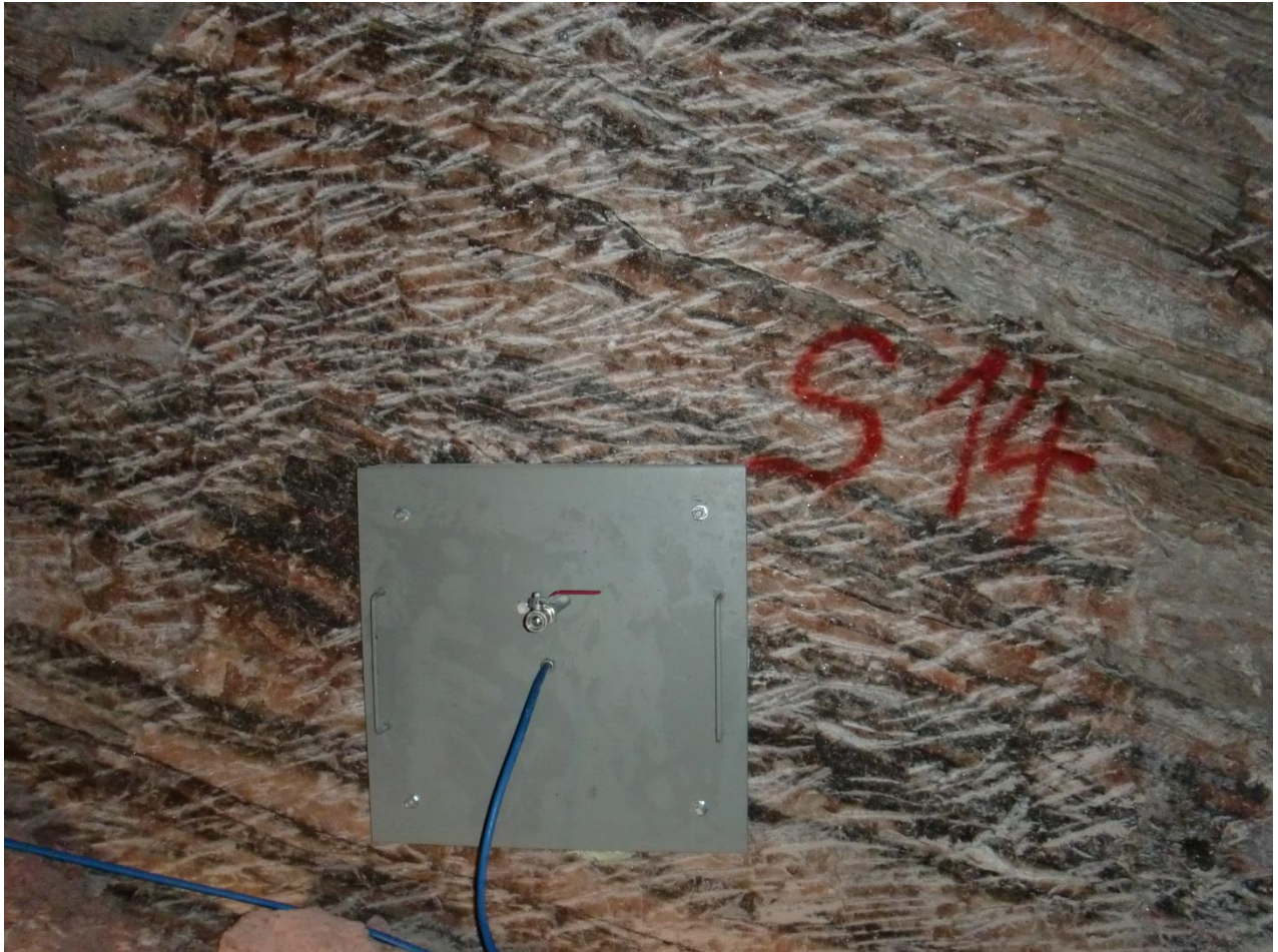
figure 3: seismological measuring site in the mine with mounting and isolation against explosive atmosphere
